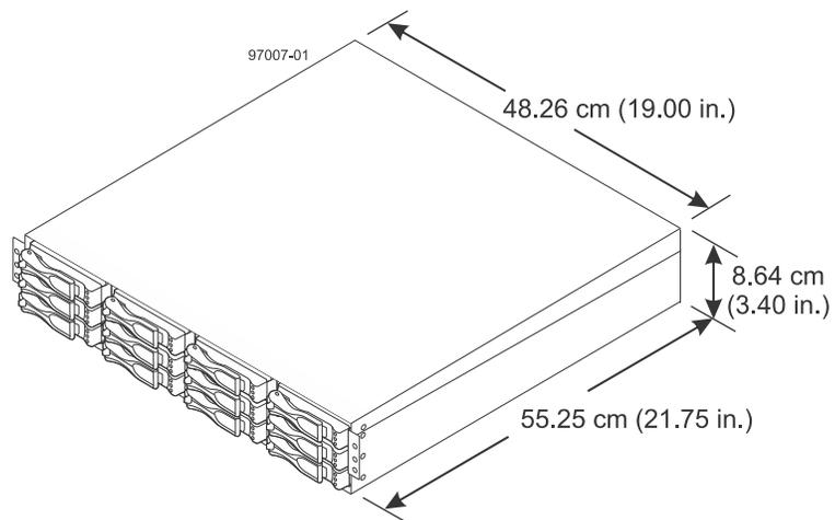
**Dimensions of the E5424 controller-drive tray or the EF540 flash array with 24 drives – front view**
