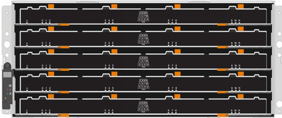
The following figure shows the back of an E2860 controller shelf:
