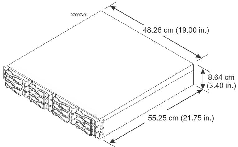
**Dimensions of the E2724 controller-drive tray – front view**
