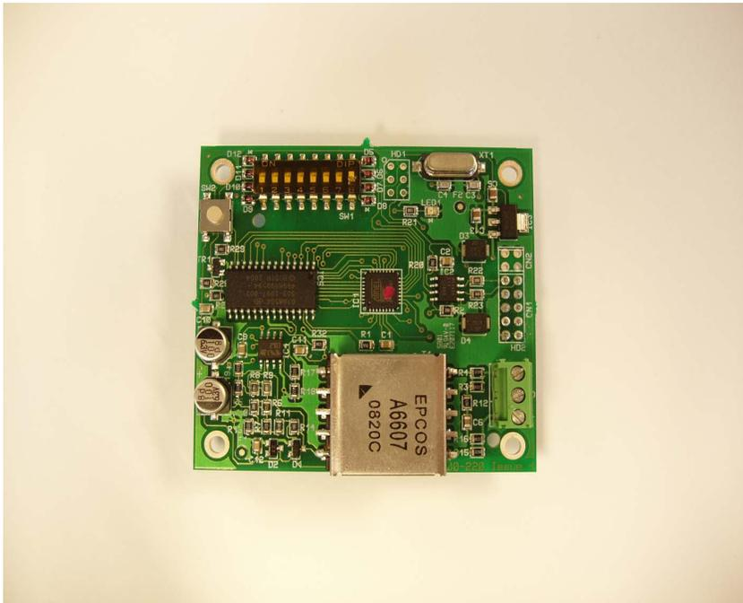
The Bi-phase converter card allows Bosch control systems with Bi-phase output to control up to eight (8) non-IR MIC400 series camera via their associated power supply units.
