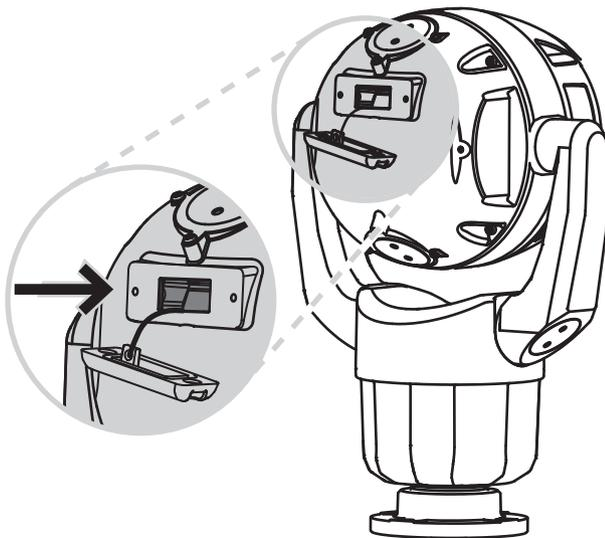
5. Push and hold the reset button for more than 8 seconds. The red LED indicator on the PCBA board will come on to show that the hardware reset started.
