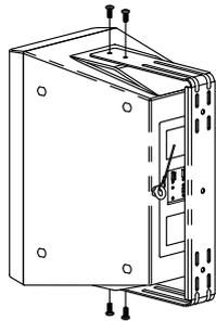
2. Install a **10-mm rated forged eyebolt** (not included) into the safety point.
