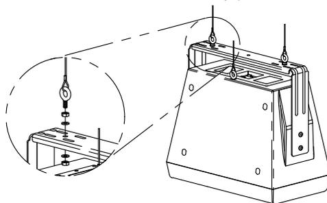
2. Install a **10-mm rated forged eyebolt** (not included) into the safety point.
