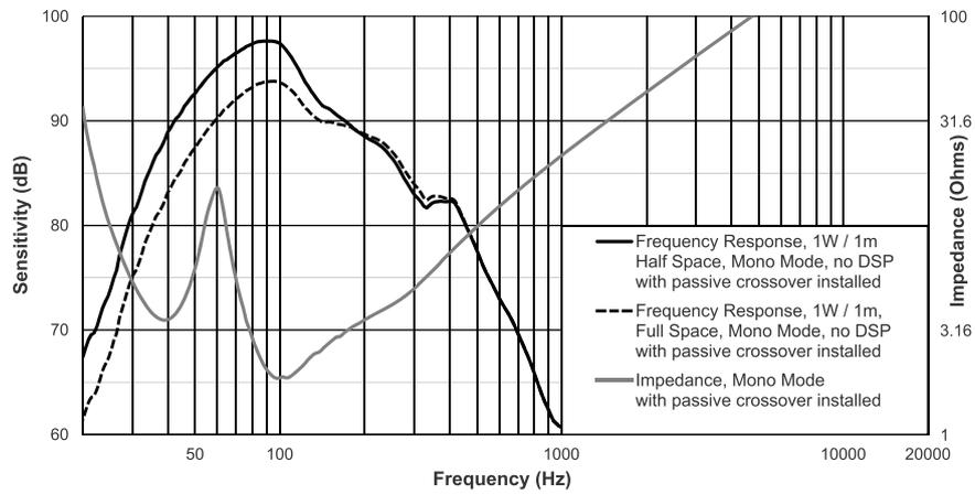
Figure 7.2: Frequency response and impedance with cross-over
