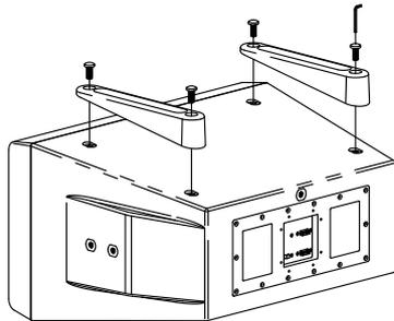
3. Attach the **mounting point covers** on the U-bracket mounting points.
