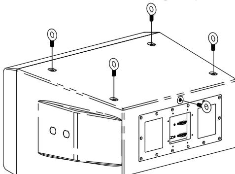
6. Install a **10-mm rated forged eyebolt** (not included) into the safety point.
