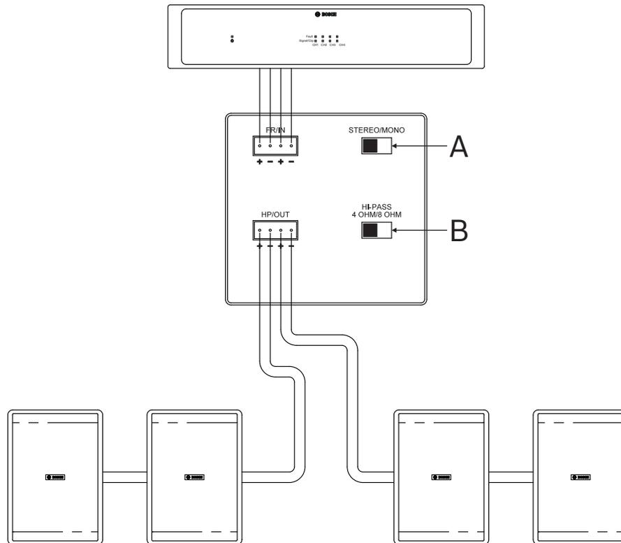
Figure 5.4: Stereo configuration 2
