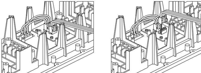
3. Connect the **transformer input panel**.
