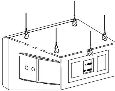
8. Secure the **subwoofer** from the safety eyebolt using rated fittings and steel cable.
