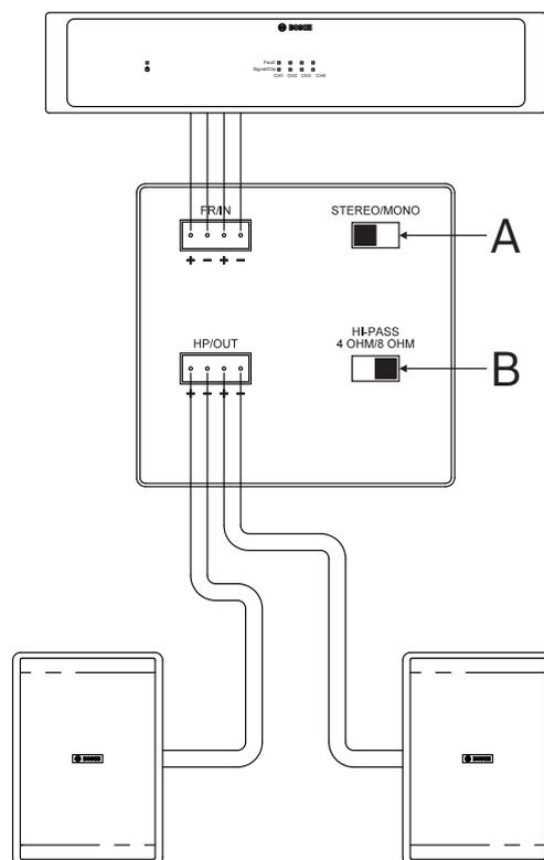
Figure 5.3: Stereo configuration 1
