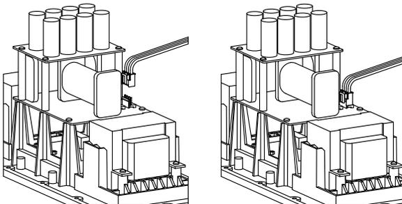
4. Install the **transformer input panel**.
