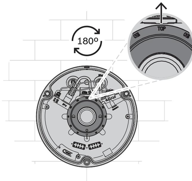
2. Put the camera cover on the camera base in the right orientation.
