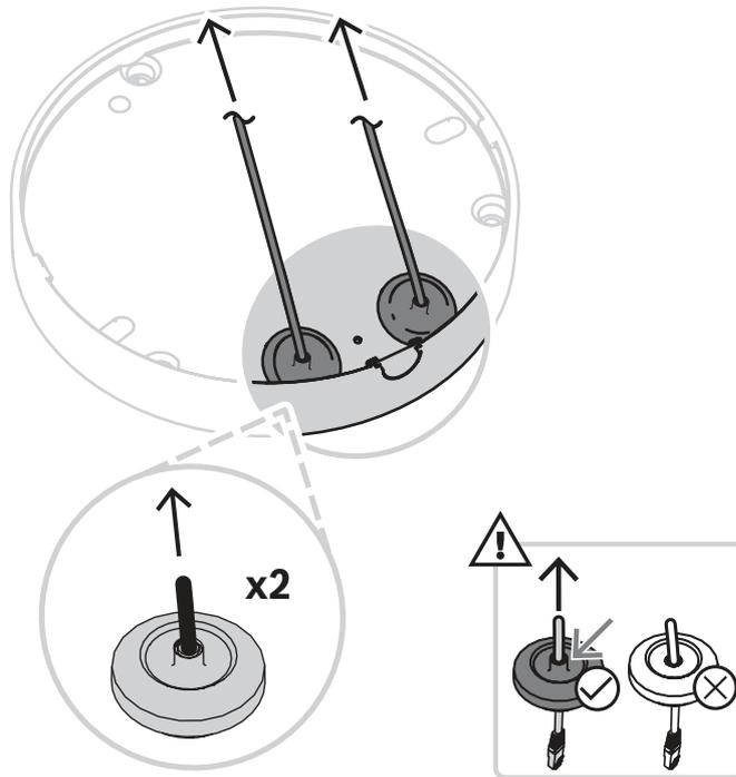
7. Connect the network cable to the network connector in the camera.
