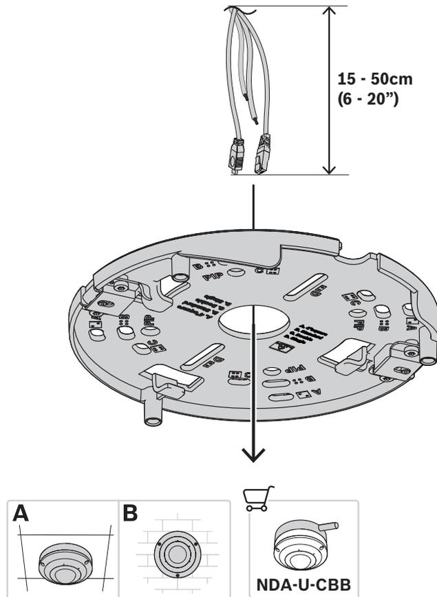
3. Pull the cable through the center hole of the mounting plate.
