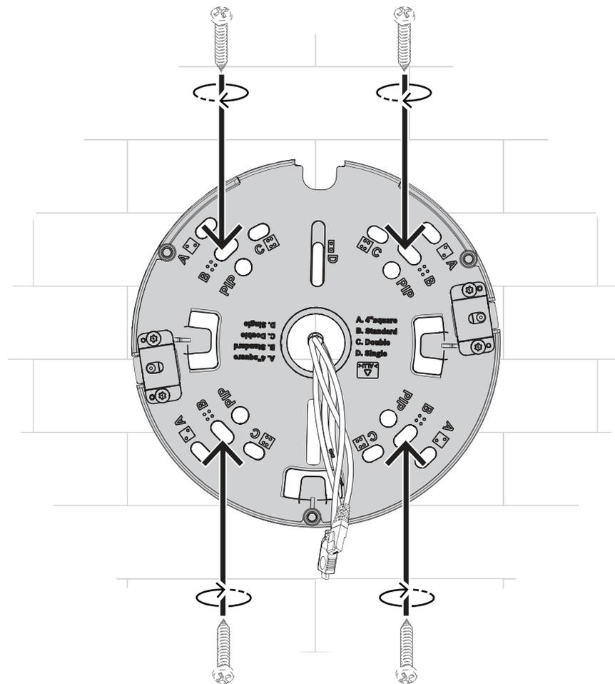
In order to ensure proper wall installation with the Bosch logo showing up straight on top, the mounting plate needs to be install as shown above.
