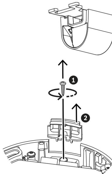
5. If there are auxiliary connections, puncture a hole in the rubber of the secondary cable inlet (2) in the camera base to put them through. The diameter of the whole must be between 5 and 8 mm (0.2 and 0.3 in.).
