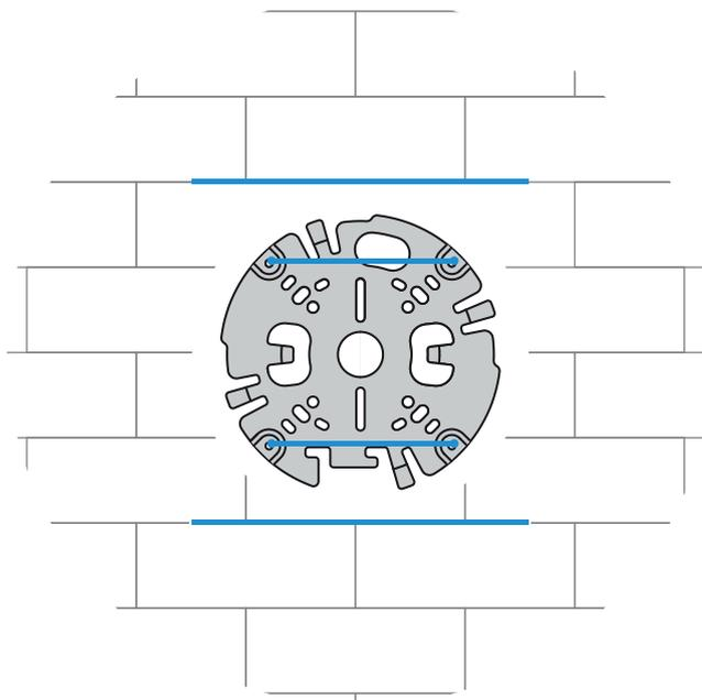
3. Drill the 4 holes with the appropriate diameter drill to support your 5-6 mm (0.2 inch) screws and plugs.
