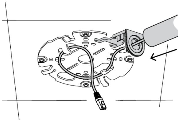
13. Install the conduit cover on the conduit plate with the bolt. Tighten the screw between 1.4 and 2 Nm (1 lbfft and 1.5 lbfft).
