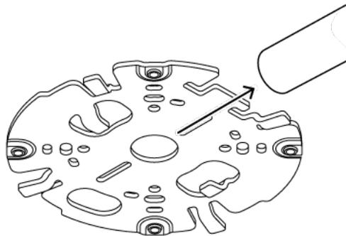
10. Drill the 4 holes with the appropriate diameter drill to support your 5-6 mm (0.2 inch) screws and plugs.
