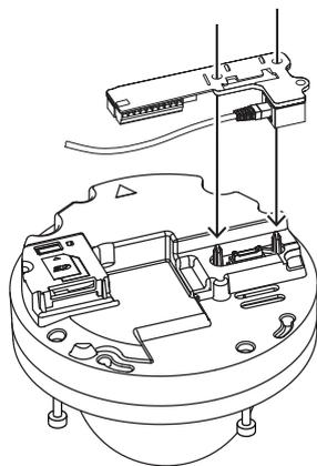
4. Connect a network cable with PoE or a 24V AC / 12-26V DC cable to power the camera module.
