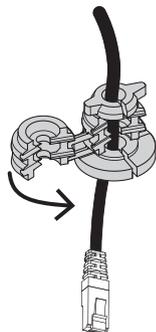
4. Grab the camera base with both hands and push the grommet into the network cable inlet with both thumbs on the opposite sides of the network cable.
