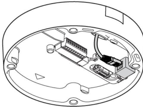
8. If required, do a loop with the cable on the hooks of the mounting plate.
