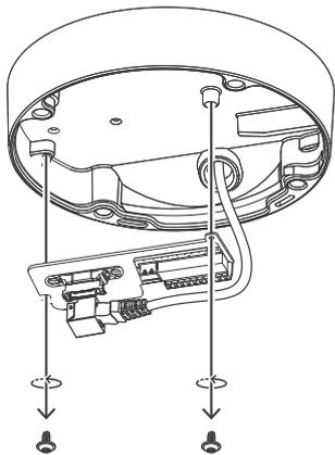
3. Attach the connection PCB to the camera module.
