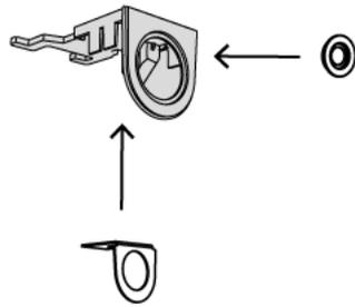
6. Put the cable through the hole of the conduit plate.
