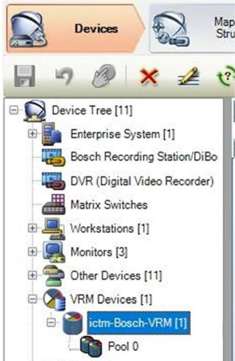
5. A pool should be automatically created under the VRM device you just added. If not, right-click the VRM device and select Add Pool.
