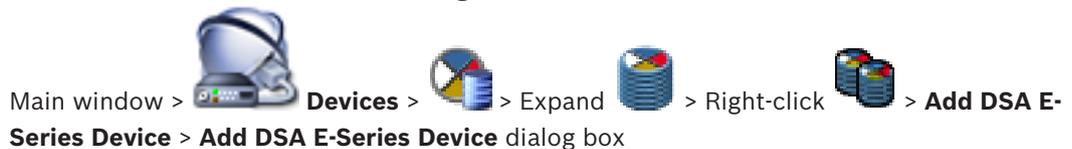
Allows you to add a DSA E-Series iSCSI device. This device type has a management IP address different from the IP address of the iSCSI storage. Via this management IP address the device is automatically detected and configured.
