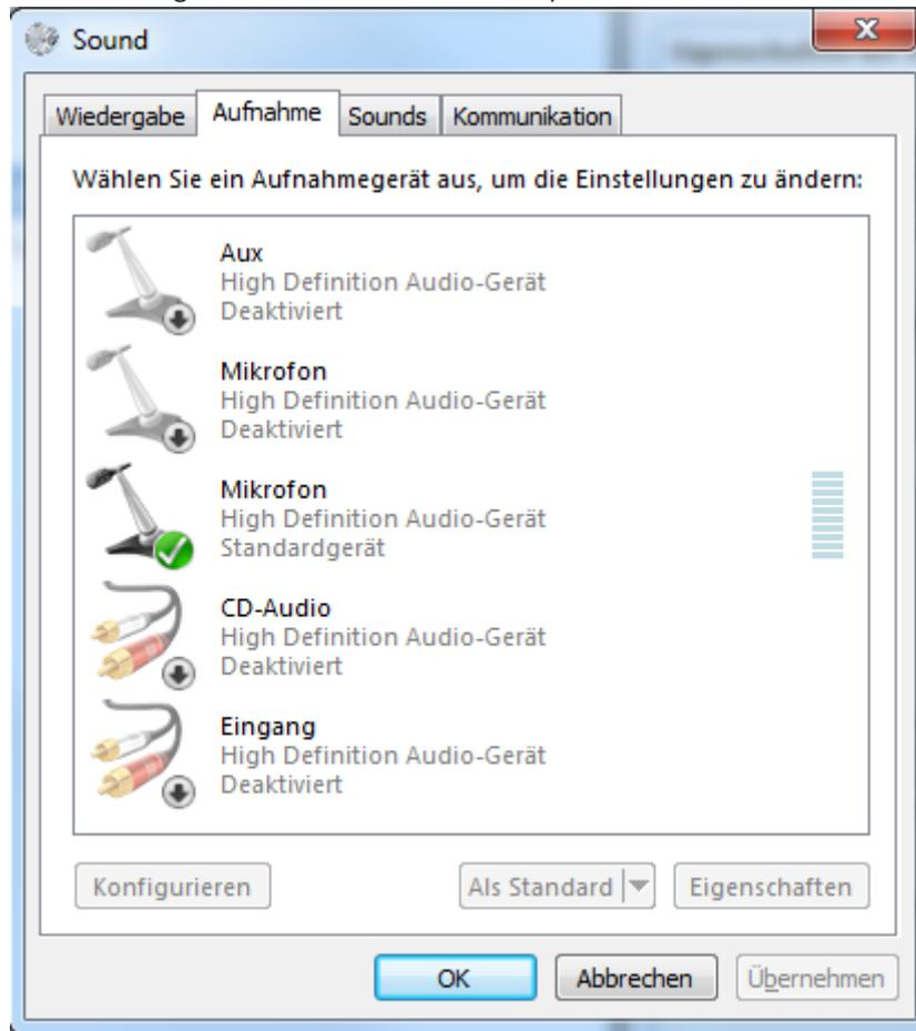
If you change the setting from stereo mix to microphone after the first start of Operator Client, the setting is overridden after the next start of Operator Client. We recommend to use a headset instead of a microphone-loudspeaker combination to avoid acoustic feedback.
