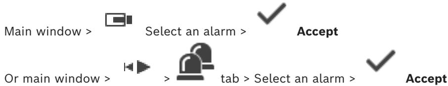
The alarm image window displays live or instant playback video from a camera, maps, documents or map viewports to be displayed in case of an alarm. The alarm image window is displayed automatically if the incoming alarm has a higher priority than the live or playback image window. The priorities are configured in the Configuration Client.
