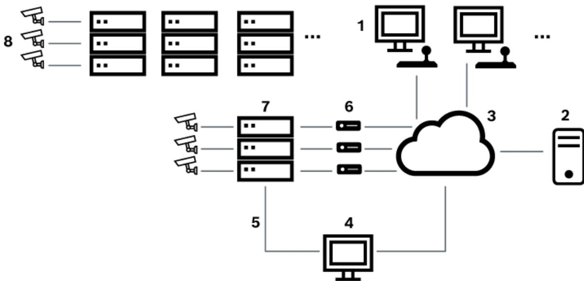
**Figure 6.5:** Bosch Allegiant system extended with Satellite switches
