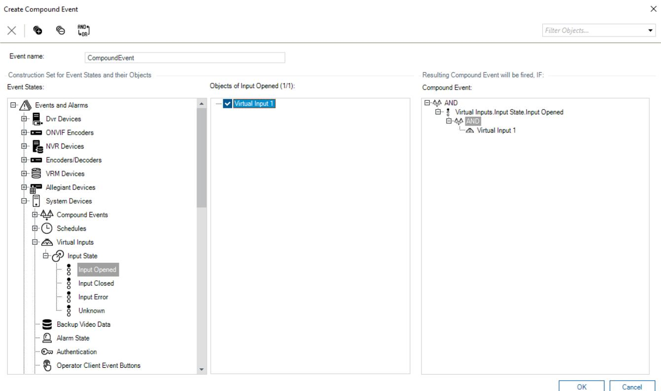
The screenshot shows the 'Create Compound Event' dialog box. The 'Event name' field is set to 'CompoundEvent'. The 'Event States' field is set to 'Input State'. The 'Objects of Input Opened (1/1):' field contains 'Virtual Input 1'. The 'Resulting Compound Event will be fired, IF:' field shows a tree view with 'AND' selected, and 'Virtual Inputs.Input State.Input Opened' and 'Virtual Input 1' as children. There are 'OK' and 'Cancel' buttons at the bottom right.
