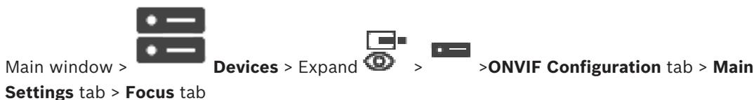
Depending on the device model you can configure here parameters for the focus. This page allows for moving the lens in an absolute, a relative or in a continuous way. Focus adjustments through this operation turn off the autofocus. A device with support for remote focus control usually supports control through this move operation. The focus position is represented with a certain numeric value. The state of the focus can be one of the following:
