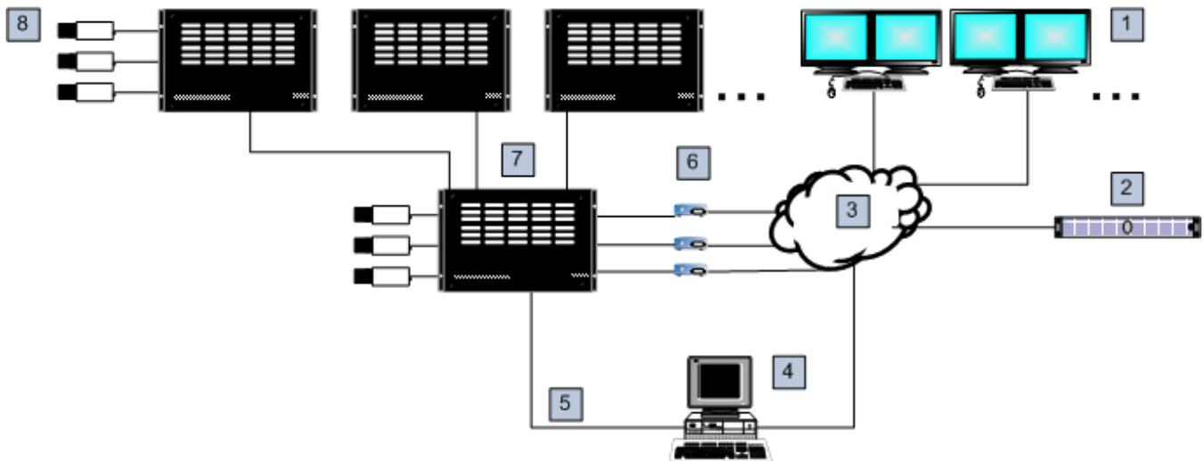
Figure 5.5: Bosch Allegiant system extended with Satellite switches
