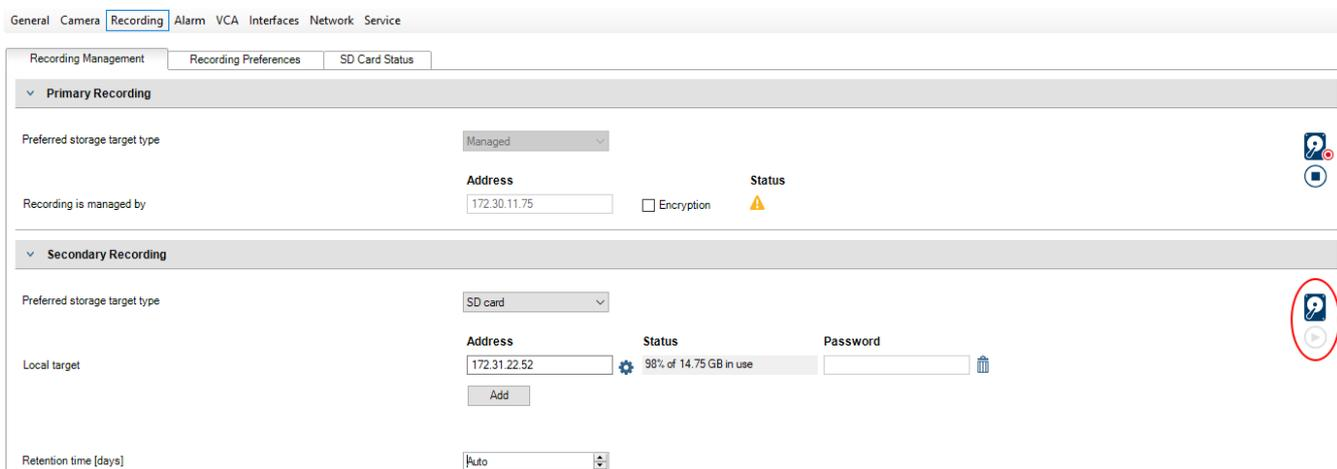
The ANR function only works on encoders with firmware version 5.90 or later. Not all encoder types support ANR even if the correct firmware version is installed.
