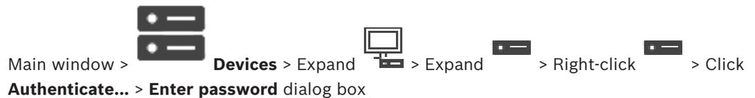
To enable the access of a password protected encoder to a decoder, you must enter the password of the user authorization level of the encoder as the destination password in the decoder.
