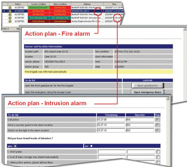
Alarm-dependent action plans or workflows provide detailed event-dependent information such as standard operating procedures, live images, control buttons, etc. to the operator. Simply create and assign one action plan to each possible alarm type in your system, e.g. fire alarm, access denied, technical alarms, etc.
