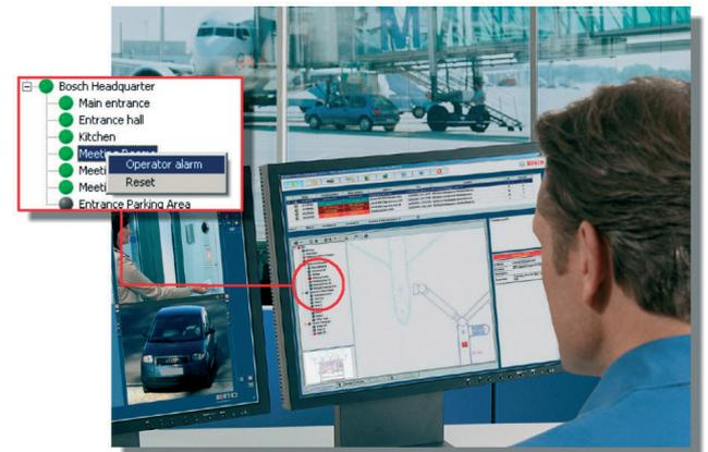
The **Operator Alarm** feature allows an operator to trigger an alarm manually from the location tree, for example, if informed by telephone of a dangerous situation. Such manual alarms are processed in the same way as those triggered by a detector: that is, the associated documents are displayed and all steps taken are recorded in the event log for thorough post-event investigation.
