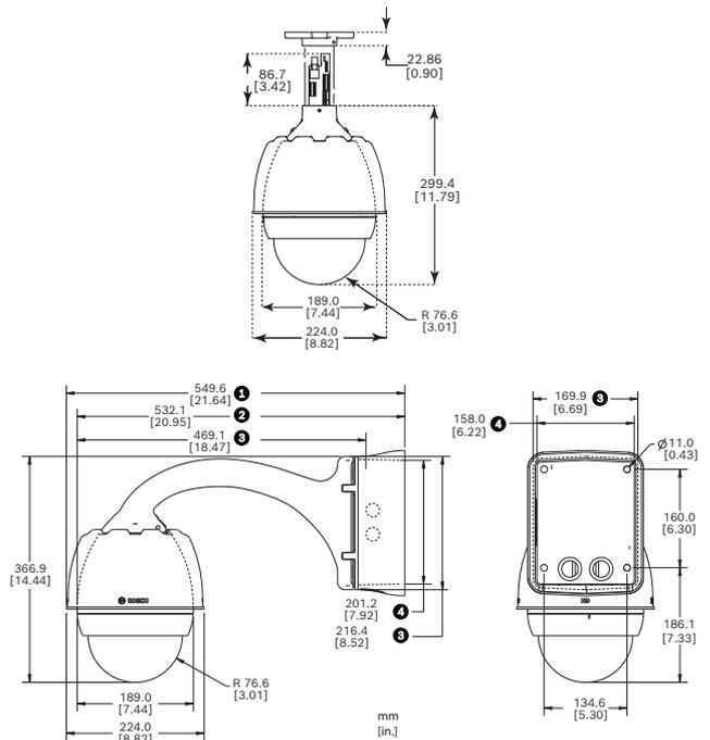
Fig. 1: Dimensions, AUTODOME7000 pipe mount, pendant mount
