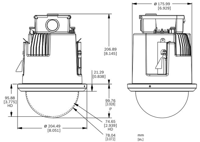
Fig. 2: AUTODOME 7000 series In-ceiling
