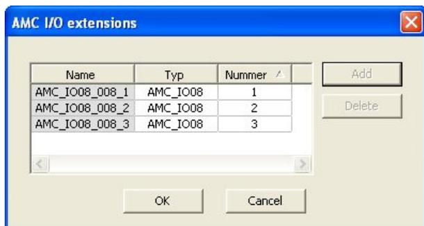
Extension boards are numbered 1, 2 or 3 as created. The numbering of the signals begins for each board at 01. The signal number in combination with the board number provides a unique identification. The signals of the extension boards can also be seen on the tab of the AMC to which they belong.
