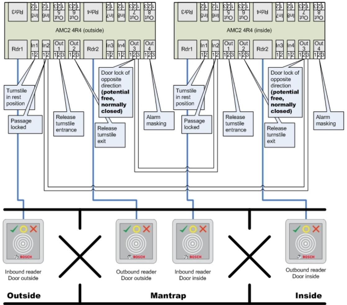
Connections to the door locks for the opposite direction ensure that only one of the turnstiles can be opened at any one time.
