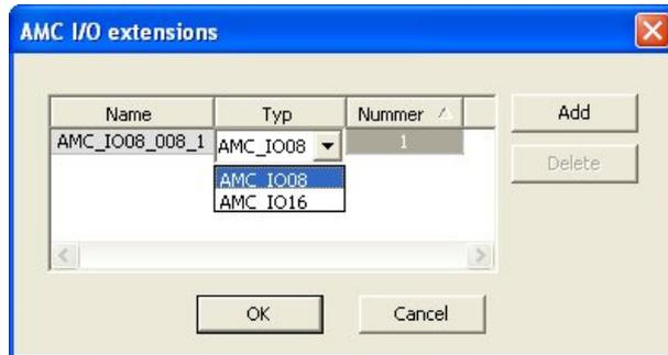
You can connect up to three extensions to one AMC. A mix of the two variants is possible. Click **Add** to create more list entries. These can all the column entries can be customized.
