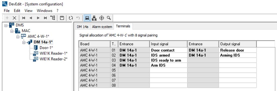
2. Select the line corresponding to the terminal that you want to use for the input signal.
