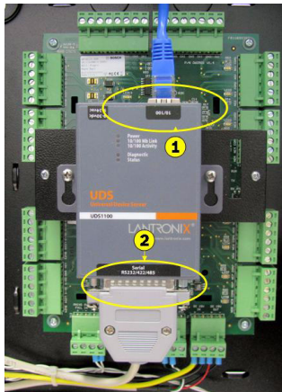
Figure 2.5 Network cable and serial cable connection points
