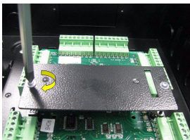
Figure 2.3 Mounting plate with the screw direction
