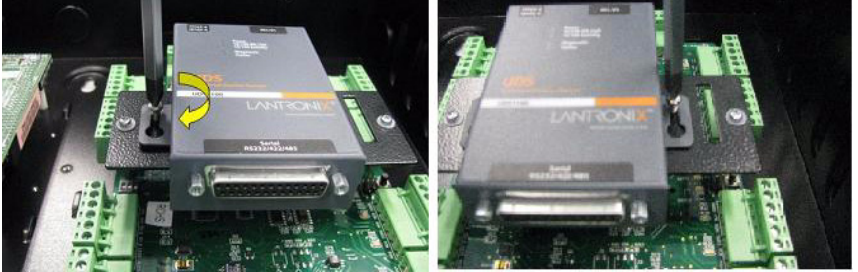
Figure 2.4 Converter mounted on plate with screw directions
