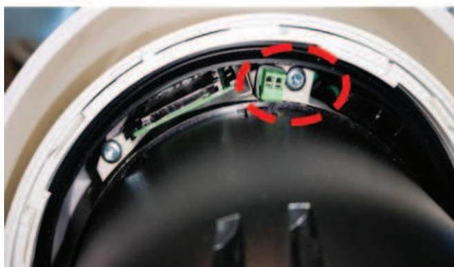
5. Create a loop with conductive wire on the connector to cause a short circuit in the two (2) terminal pins. Hold the loop on the terminal pins for more than ten (10) seconds. The red LED indicator on the PCBA board flashes to show that the short circuit set the factory defaults of the camera.
