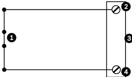
**Figure 14.4:** N.C. Normally Closed Non-supervised Connections
