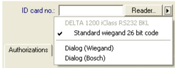
In the case of input readers with Hitag, Legic or MIFARE read-processes the actual reader entry is generated and can be selected from the list directly.
